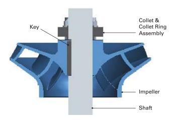
Impellers are fixed to impeller shaft with collet ring and collet along with key.
