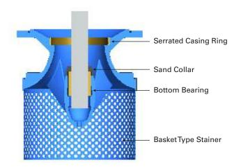
Provision of bottom bearing helps to provide support to the impeller shaft, enabling the impeller to run between bearings. Serrated wear rings ensure less metal contact and sustained efficiency. Basket type strainer avoids entry of undesired size of solids in the pump.
