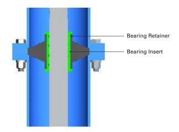
Bearing retainer is sandwiched within spigot of column flanges. Fluted bearing insert supports line shaft and is lubricated with pumped water.
