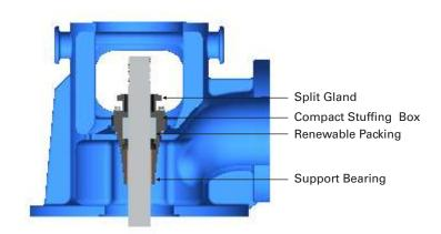
Stuffing box packing is provided as a standard supply, stuffing box is provided with inbuilt bush which support head shaft. Cast discharge head provide more rigidity and stability to the pump.
